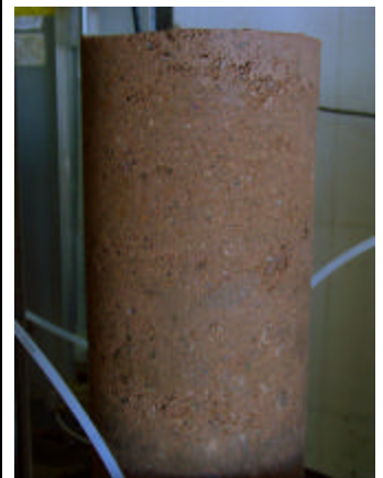
Remolded Triax Sample by compaction.; 6"d x 12"h; six 2" lifts; each lift batched to required gradation
