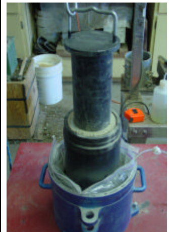
Remolding of gravel by vibratory table. 6"d x 12"h; six 2" lifts; batched to required gradation
